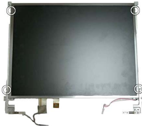
Fig. 26 Removing hinge screws
